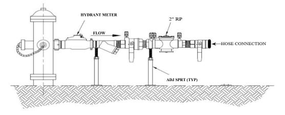
Note: A Backflow Assembly must be supported. Any damages to the Meter and/or Hydrant will be deducted from your deposit.
