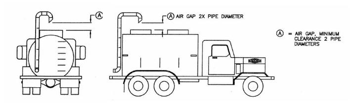
**Backflow -** If connecting a hose directly from a Hydrant without proper Air Gap, a Backflow Assembly (RP) is required
